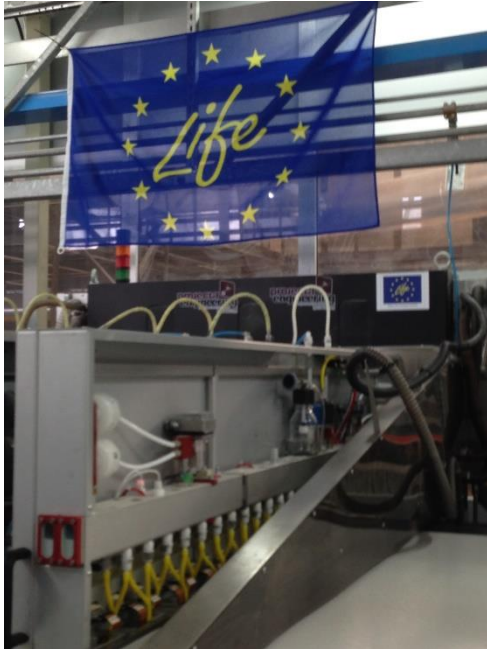
Fig. 2 - In the picture the detail of a print head bar containing the formulation based on \text{TiO}_2
