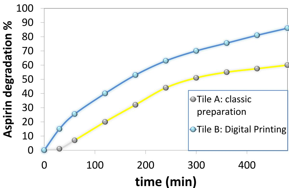
The graph shows the aspirin degradation in contaminated water using Active tiles under irradiation by UV light.
